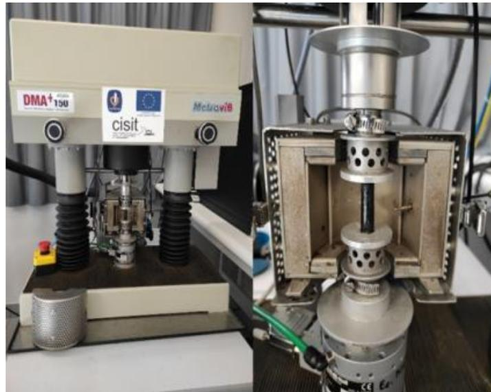
Appareil DMA-module (compression-traction)
